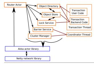
Figure 14. Hyflow2 system diagram
